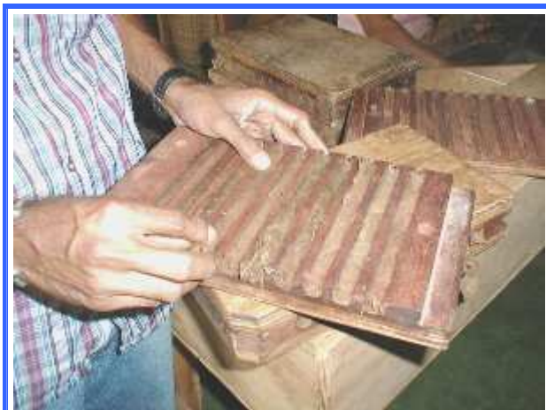
The cigar factory in La Pintada has a 20 year history in the community and produces fine, inexpensive cigars. The above photo shows the cigars being put into a cigar mold that is later covered by a lid and then put on top of other molds -- all of which are pressed by a large vice.
